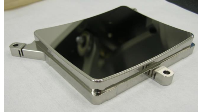
Complex shape with tolerances 50-100nm
